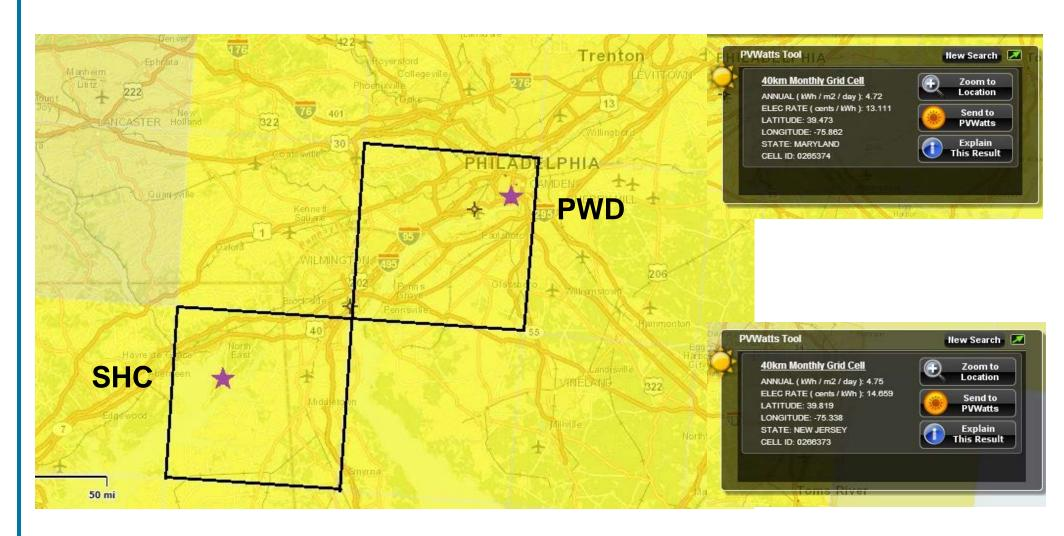
It is crucial to refine PV energy estimating programs to account for site differences at specific geographic locations. Currently, solar radiation and albedo are averaged at 40km<sup>2</sup> cell resolution. As seen on the left, both research sites are incorporated into neighboring grid cells.
