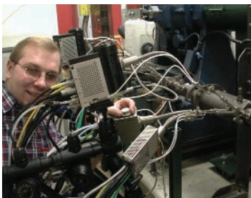
Masters student Justin Delecki inspects the sampling heads of the newly commissioned Fast Gas Analyzers from Combustion Ltd, UK
