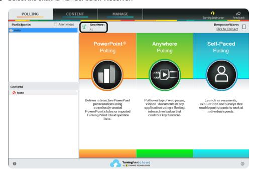
4 Select a new channel (1 - 82 for RF and RF LCD; 1 - 74 for XR and NXT) from the Receiver drop-down menu.
