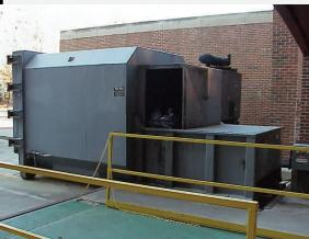
Never reach inside the hopper of a compactor, use a long stick if needed
