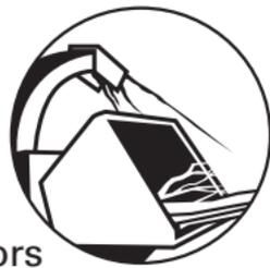
Chipper machines cut tree limbs into small chips. Hazards arise when operators get too close to, or make contact with, the chipper. Contact with chipper operating components (blades, discs or knives) may result in amputation or death. Operators may also be injured by material thrown from the machine. To minimize these hazards, use appropriate engineering and work practice controls, including operator training.
